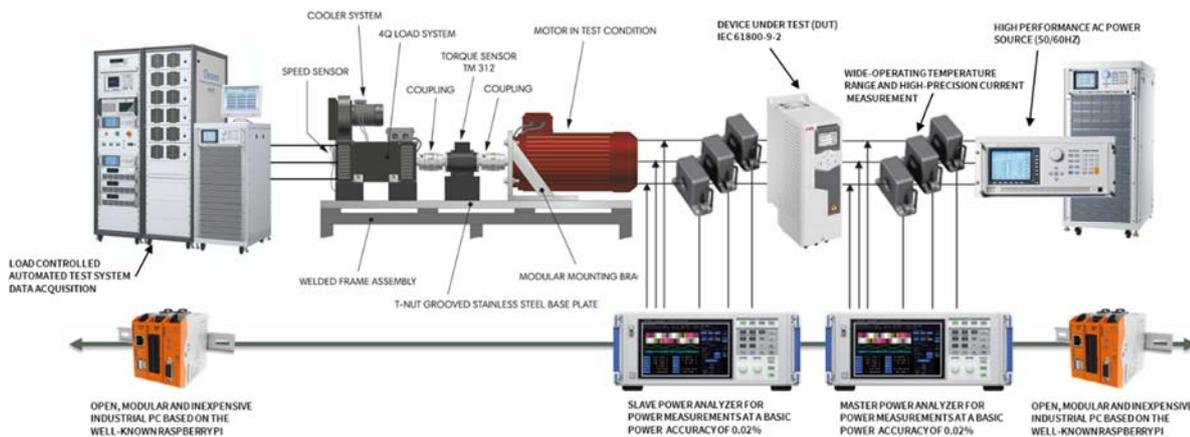
*Automated efficiency testing test bench. In addition to conventional motor tests involving the test object, load machine and torque measurement, standard efficiency testing requires a high-quality power source, a winding ohmmeter, a power analyzer and a test automation system.*
