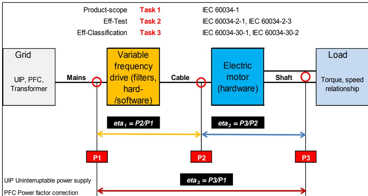
**Figure 5** The scope for measurements and efficiency classes electric motors and variable frequency drives (Source: IEC 61800-9, draft 2013)
