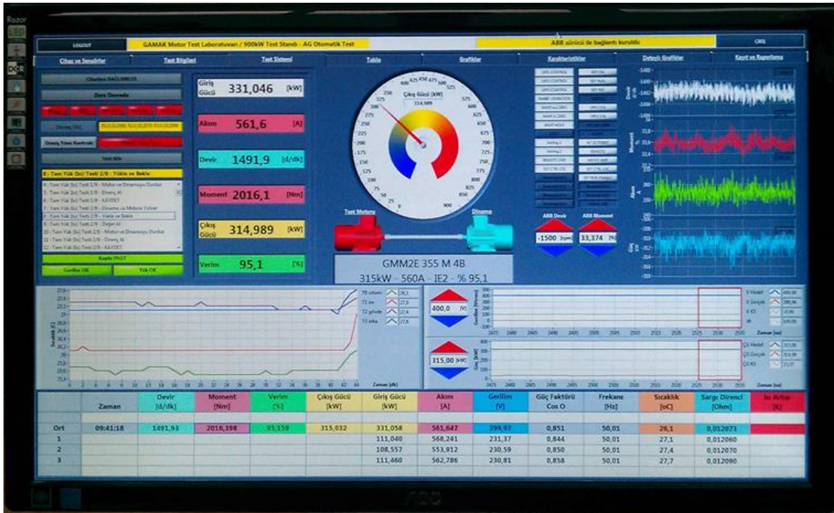
Figure 13 Programmed testing sequence and automatic data acquisition. Measurement of 315 kW 4-pole IE2 motor with variable torque. (Source: Gamak Motors, Istanbul, 2013)
