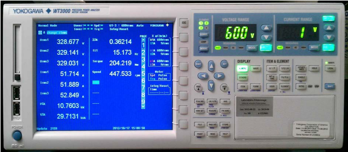
Figure 12 Yokogawa WT 3000 Precision Power Analyzer in a variable frequency efficiency measurement of the set-up in Figure 11 at the motor testing laboratory of Hydro Quebec near Montreal (Source: Pierre Angers 2013)
