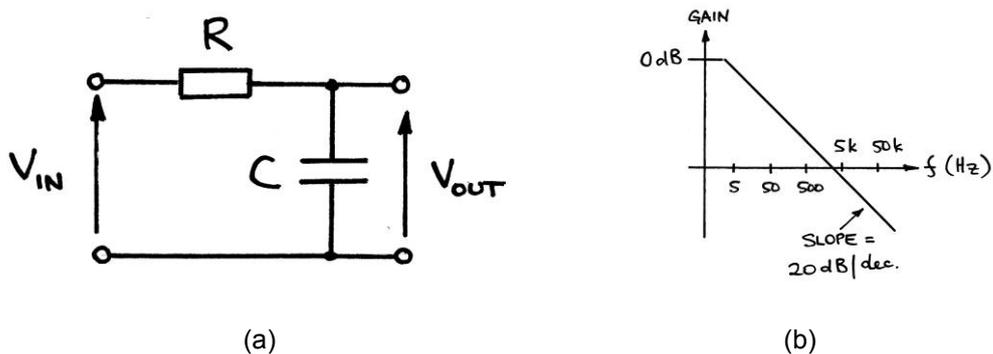
**Figure 2:** (a): A single pole passive R-C network accurately integrates signals whose frequency components are significantly greater than the cut-off or corner frequency. (b): Passive integrator frequency response characteristic
