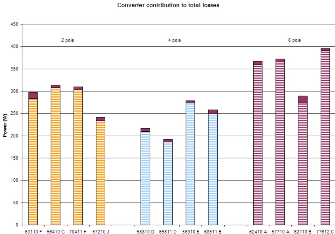
**Figure 4:** No-load loss measurements on 2, 4 and 6 pole motors with essentially sinusoidal and converter supply, the sections at the tops of the bars representing the additional losses under converter supply. These measurements were facilitated by the use of a flux voltmeter to adjust the motor supply voltages to comparable values
