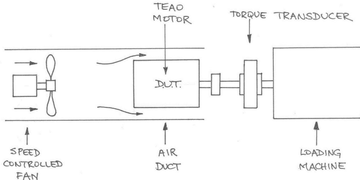
**Figure 7:** Suggested TEAO efficiency measurement set-up
