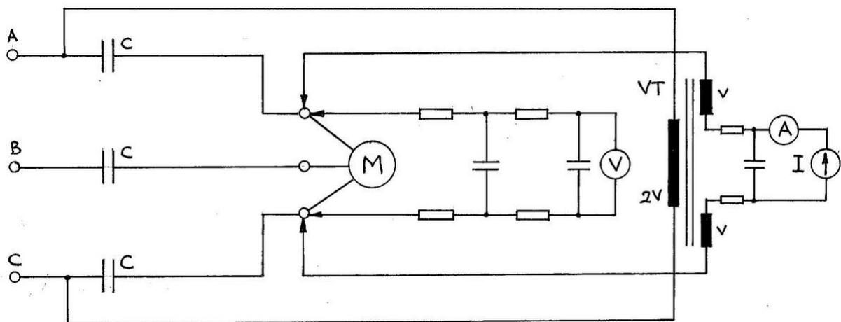
**Figure 6:** On-line resistance d.c. resistance measurement principle
