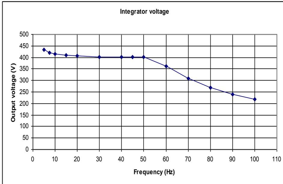
**Figure 5:** Flux voltmeter ('Integrator voltage') readings vs. frequency for a converter set to produce a 'reference converter' waveform at a fundamental output frequency of 50 Hz
