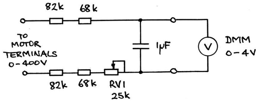
**Figure 3:** Practical (balanced) flux voltmeter according to the above design. The variable resistor allows adjustment.
