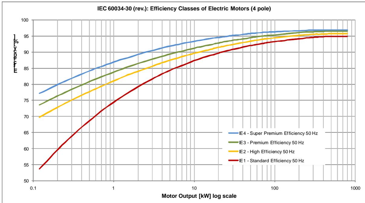
**Figure 6 IEC 60034-30 Efficiency Classes: Planned revision with classes from IE1 to IE4 and output sizes from 0.1 kW to 800 kW (source: IEC TC2 WG31, 2011)**
