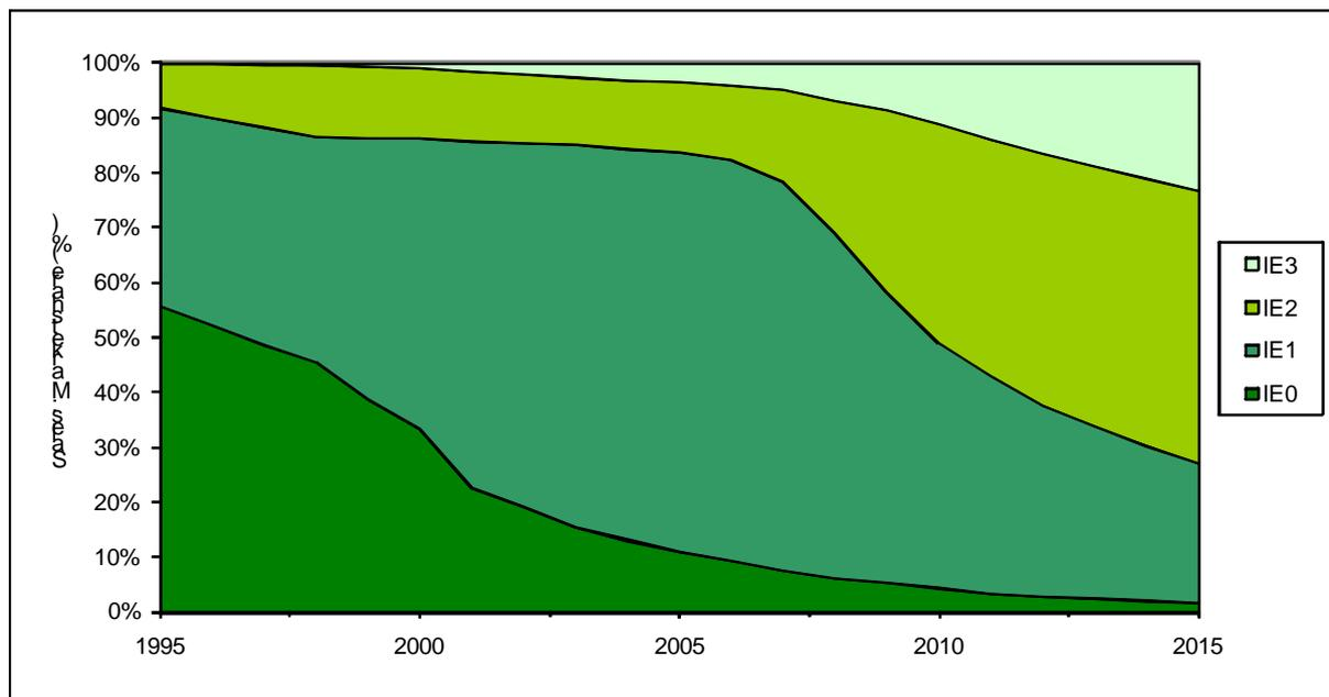
**Figure 3 Market shares of global electric medium sized motor sales shift from low to premium efficiency motors. IE1 to IE3 refer to Table 4, IE0 depicts former low-efficient Eff3 class (source: Brunner, Jakob et al. 2009, [10])**
